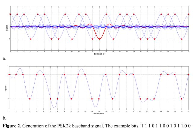
The horizontal spacing of the bits (1.0 in the figure) corresponds to 0.5 ms because of the bitrate of 2000 bits/s. The PSK2k-signal is an analog signal. But the PSK2k program generates it at a user-chosen sampling rate. If the sampling rate is 32000 for example, the spacing is 16 samples.
