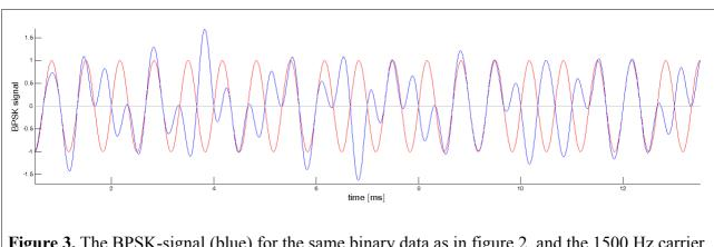
**Figure 3.** The BPSK-signal (blue) for the same binary data as in figure 2, and the 1500 Hz carrier (red).
